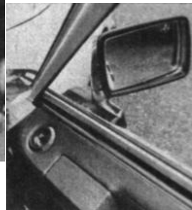
Below right: The door mirror is electronically adjustable by means of the small control on the sill
